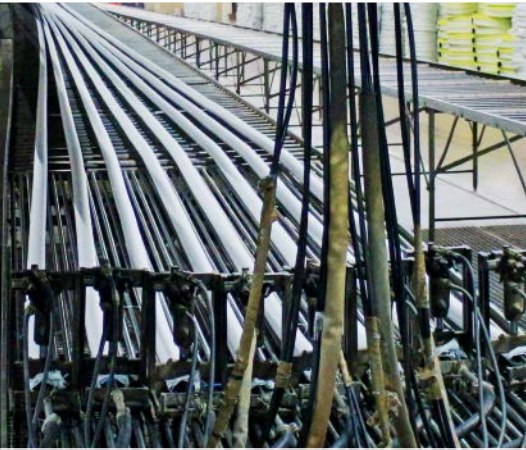
hoses during vulcanizing process
