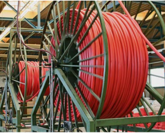
process of manufacturing endless hoses allows us to deliver lengths of more than 500 m in one section
