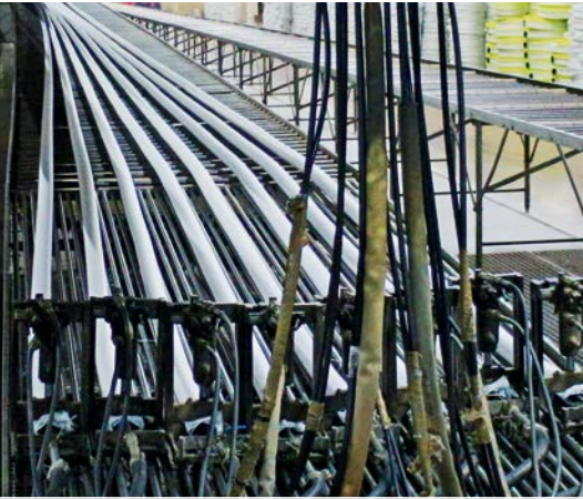
hoses during vulcanizing process
